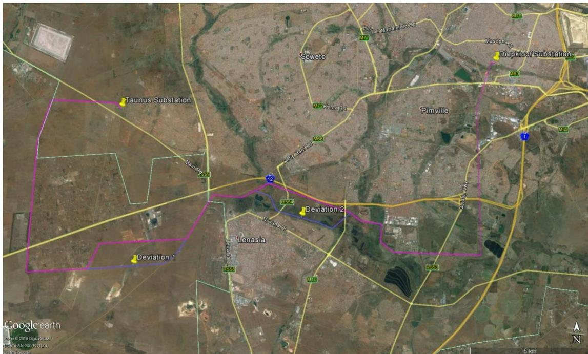
**Figure 1:** Proposed alignments for Taunus – Diepkloof 132kV. The purple line represents the proposed alignment and the blue sections the alternative alignments.
